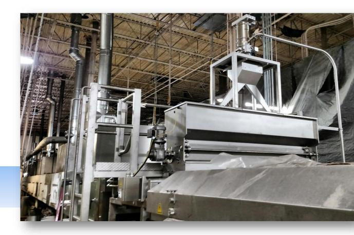
**Problem:** A customer needed to replace a portion of an existing snack food oven and upstream processing equipment to increase reliability to keep up with increased production demands. Due to quality concerns, the oven also required the ability to switch from direct-fired to indirect heating. The customer's primary goal: to increase capacity of the existing oven line.
